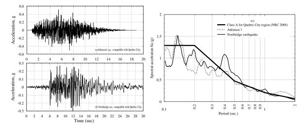
Figure 5. (a) scaled synthetic accelerograms (b) scaled Northridge earthquake to the seismicity of Eastern Quebec City. (c) Acceleration spectra for synthetic and Northridge earthquakes spectrums compatible with Eastern Quebec seismic.
