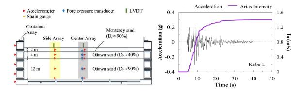
Figure 3. Schematic of the Centrifuge model and the scaled horizontal acceleration time history of Kobe-L [1].
