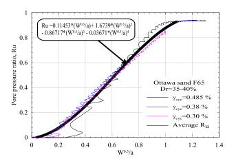
Figure 1: Ru-Ws relation after strain-controlled tests
