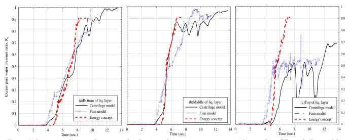
Figure 4. Comparison between the measured and estimated pore water pressure at (a) bottom (b) middle, and (C) top of the loose Ottawa sand layer.
