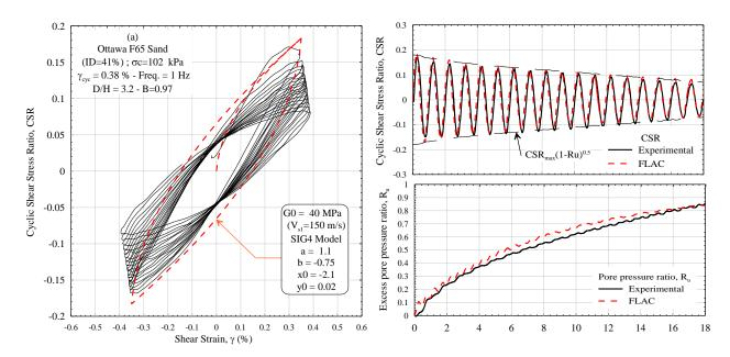
Figure 2. Typical results of TxSS test and numerical model in terms of (a) Hysteresis loops (CSR- $\gamma_{cyc}$ ), (b) CSR time history, (c)  $R_u$  time history.
