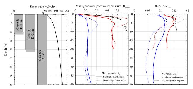
Figure 6. (a) Shear wave velocity and (b) maximum average cyclic stress ratio and generated pore water pressure ratio,  $R_u$  calculated by 1D linear analysis along depth in the uniform soil deposit by 2 earthquake motions.
