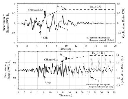
Figure 7. The cyclic response of 20.00 m deposit at 5-6 m.
